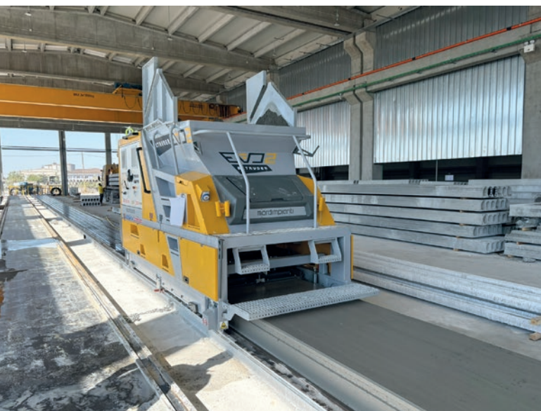
EVO2 Extruder during the casting phase
