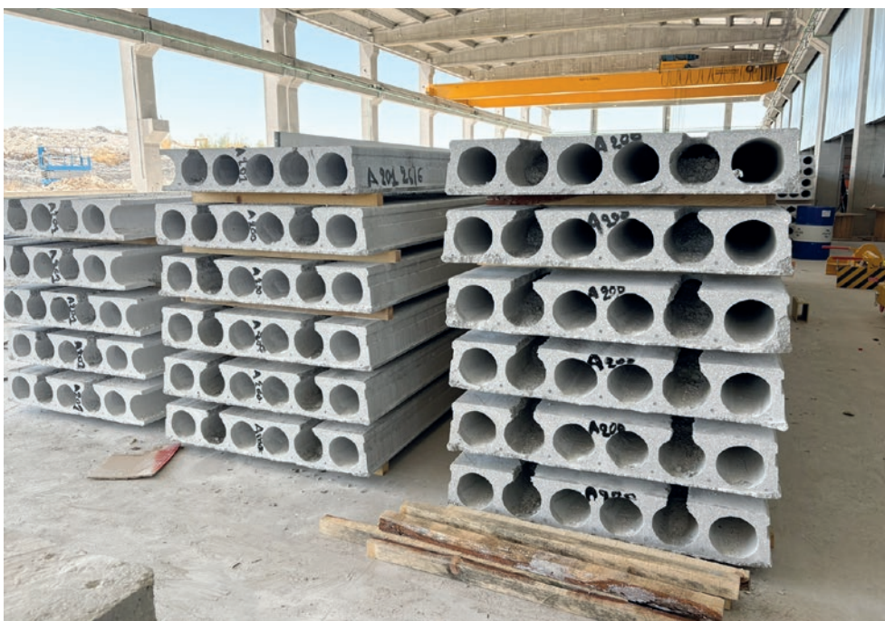
Hollow core slabs in the stockyard ready for delivery to site
