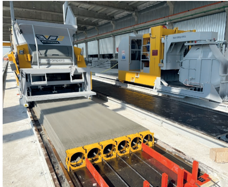
Utilising the starting plate at the beginning of the production bed to reduce waste
